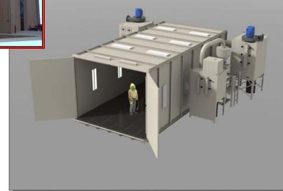
gauge steel walls and ceilings with 1.5 inch thick floor grating . Units are designed with full width work doors on one end or a thru style with doors on both ends. Cross draft or down draft air flow models available. Additional operator media delivery systems are available with complete operator safety and breathing equipment. Size of rooms are customized for the individual customer's application.
